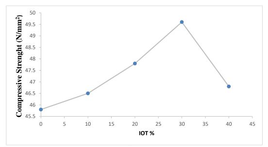
Figure 4.4: 28 Days Compressive Strength against Percentage Replacements
