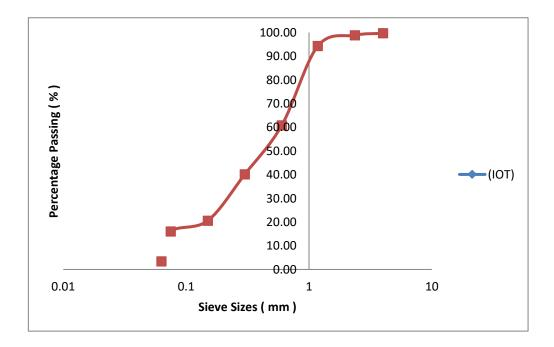
Figure 4.2: Particle Size Curve of IOT
