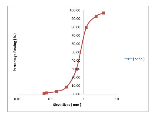
Figure 4.1: Particle Size Curve of Sand
