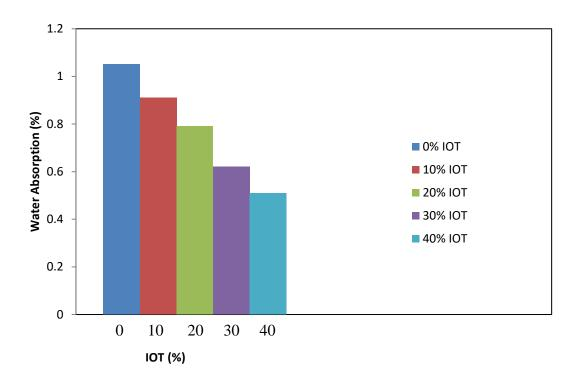
Figure 4.5: 28 Days Water Absorption
