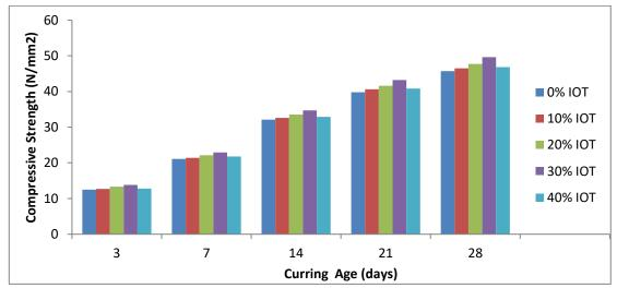
Figure 4.3: Variation in of the compressive strength with curing age
