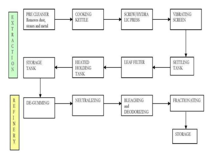
**Figure 2.1** Industrial shea butter extraction plant and refinery Source: Addaquay (2004)
