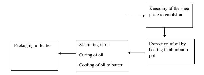
**Figure 4.1**: Flow chart of shea nut processing in Kwara and Niger States, Nigeria. **Source**: Field survey (2019).
