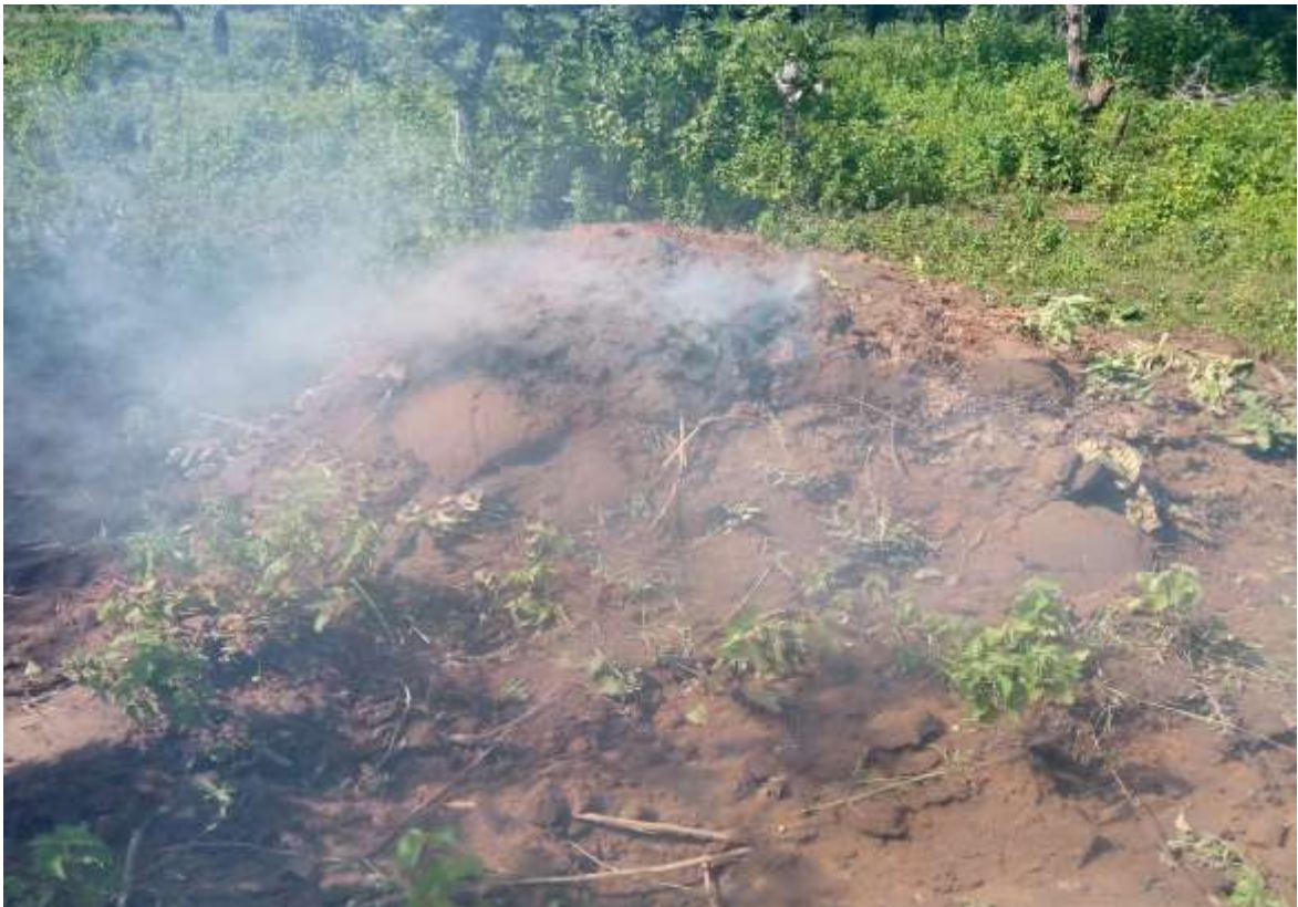
Plate II: Charcoal Carbonization Process (earth mound kiln) in Kaniyan Community
