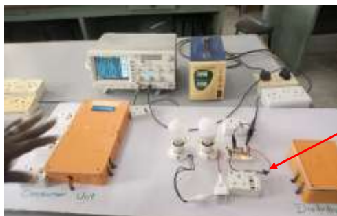
Plate 3.6: Experimental test showing Inductive load on 10Hz supply
