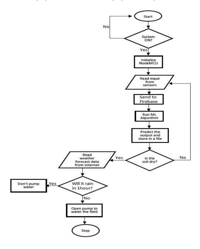
Figure 3.11: Flowchart of Autonomous Irrigation System
