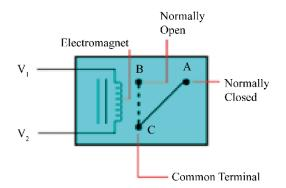
Figure 3.3: Relay Internal Diagram
