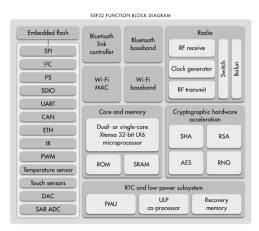
Figure 3.5: ESP32 Function Block Diagram(ESP32, n.d.)
