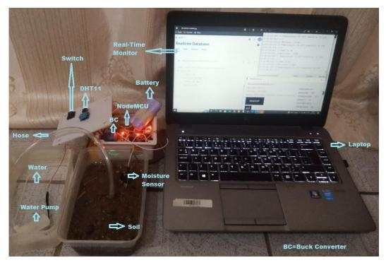
Plate I: Autonomous irrigation system setup
