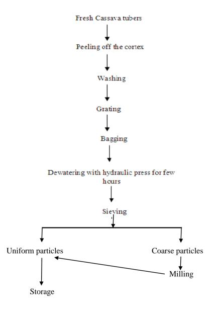
Figure 2.3: Flow Chart of garri processing operation (IITA, 2018).
