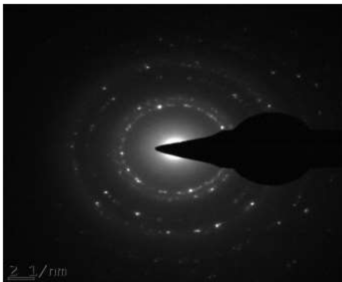
Plate V:- Selected Area of Electron Diffraction (SAED) pattern of AuNPs
