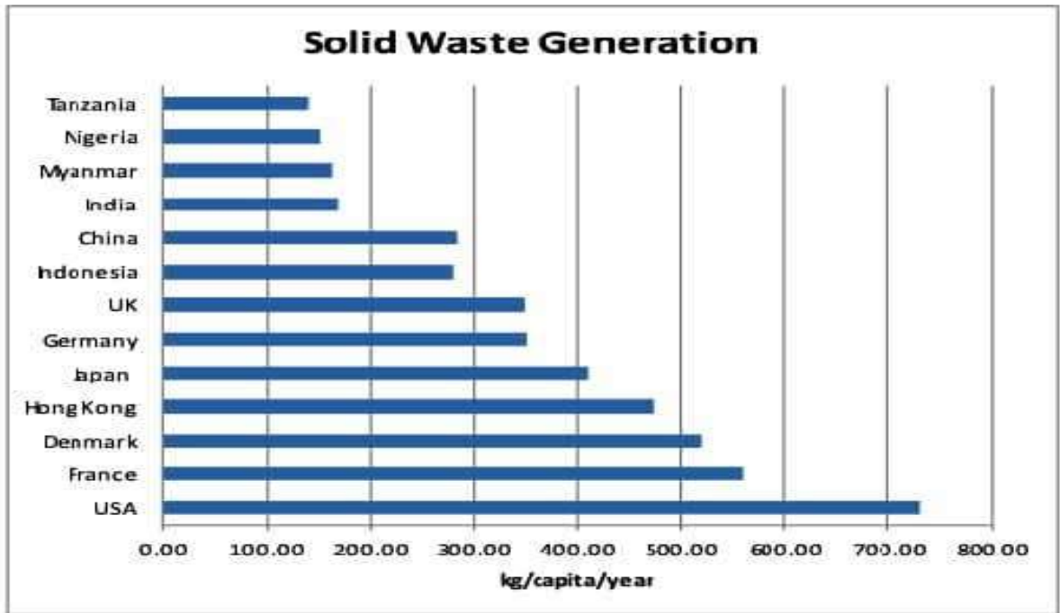
Figure 2.1: Solid Waste Generation in Selected Countries (Raw data from: Lau, 2004; WHO, 2006, Pippati,2006).
