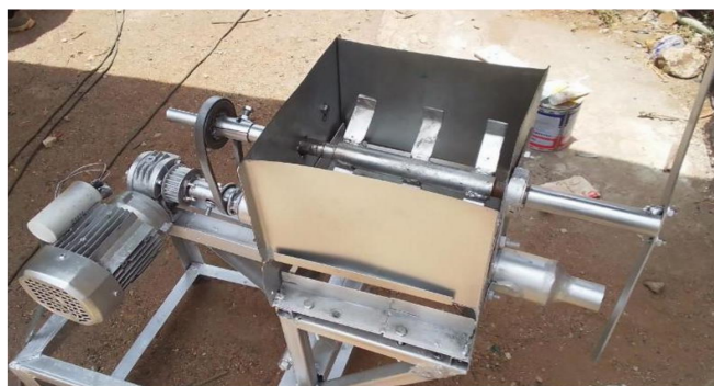
Plate XI: The Pictorial View of the Assembled Donkwa Production Machine.
