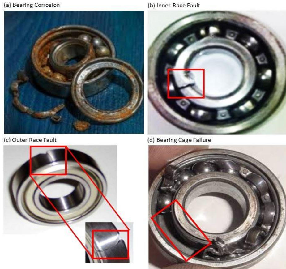
Figure 2.5: Manifestation of bearing faults
