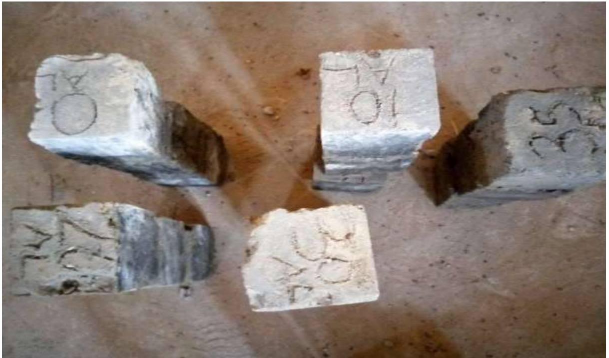
Plate VII: Concrete at 28 days of curing
