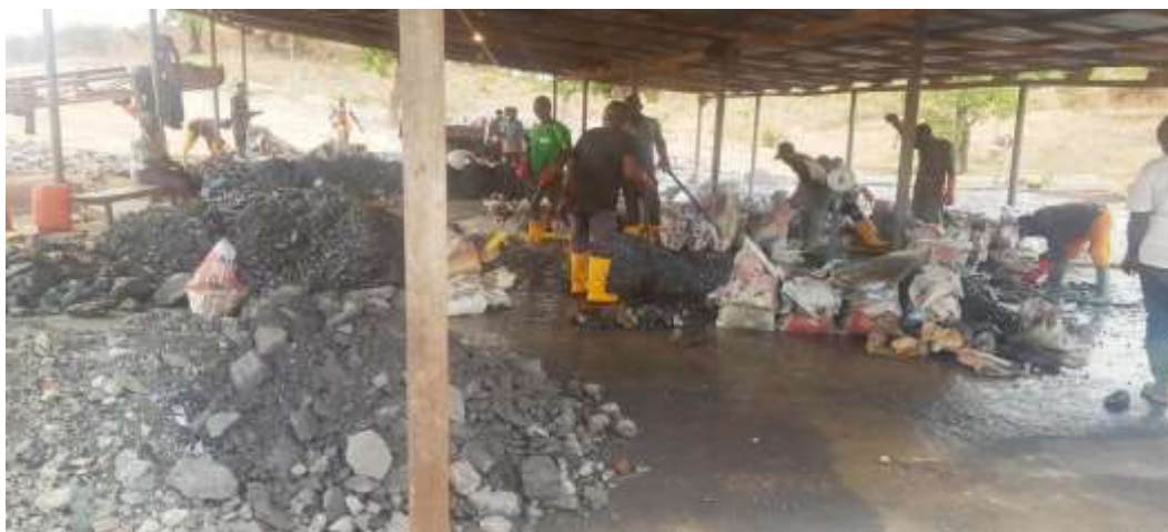
Plate XII: Mines workers sorting and washing the Pb-Zn ore.
