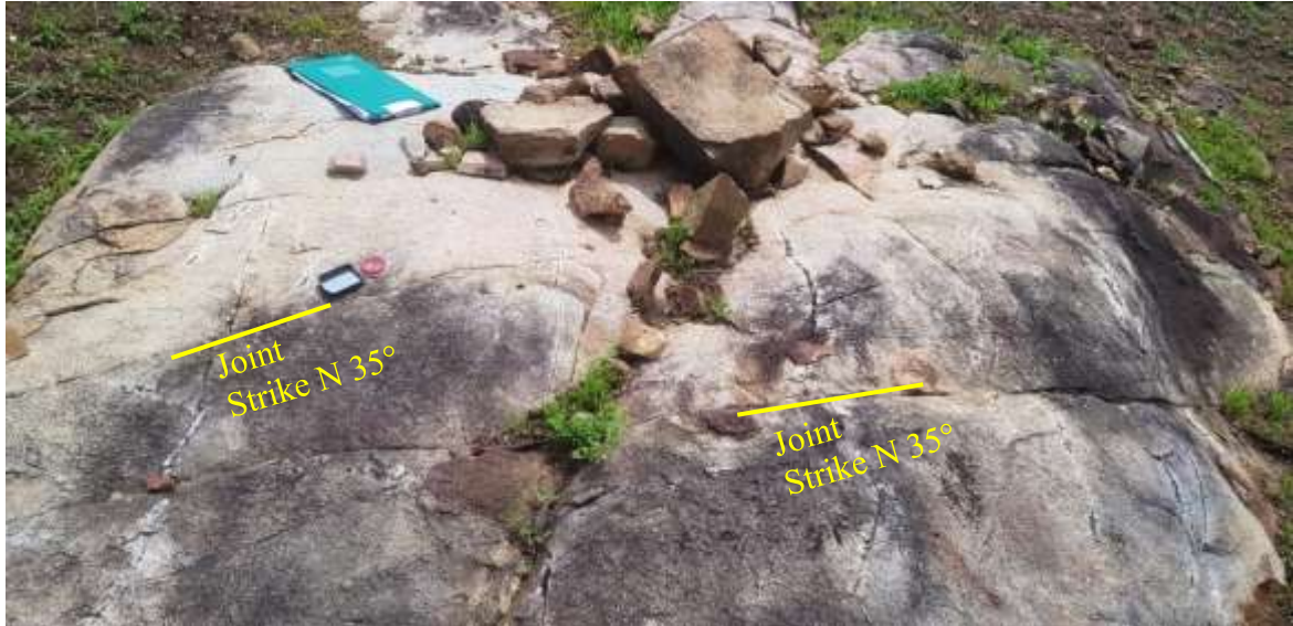
Plate III: Weathered and jointed (marked by yellow lines) medium-coarse grained biotite granite outcrop. Location coordinates (N 08° 41' 04.0", E 08° 33' 02", 210m ASL).
