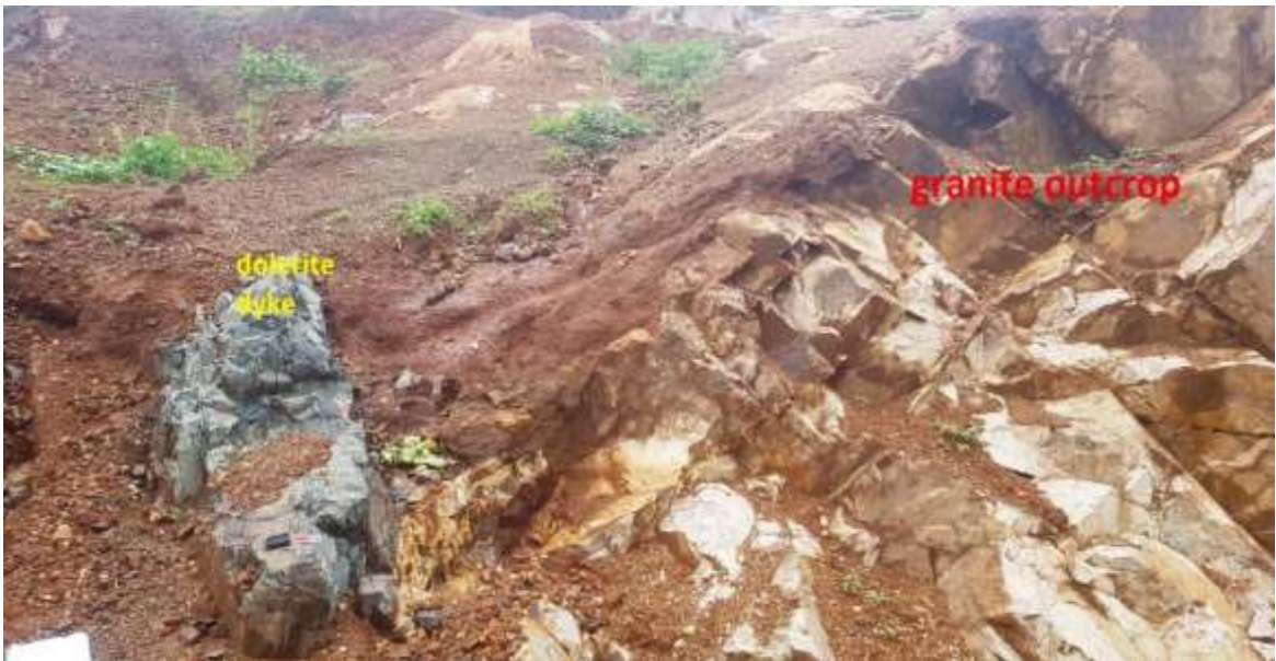
Plate VIII: Dolerite dyke 0.5m wide cross cuts highly weathered and jointed granite outcrop. (Location coordinates: N08° 42' 02.4", E08° 32' 33.9", 281m ASL)
