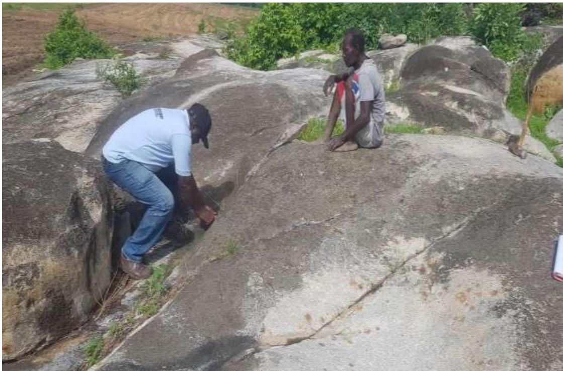
Plate XVI: Jointed and fractured granodiorite outcrop at Dinding (8°50'38.5"N, 11° 46' 10.2"E)
