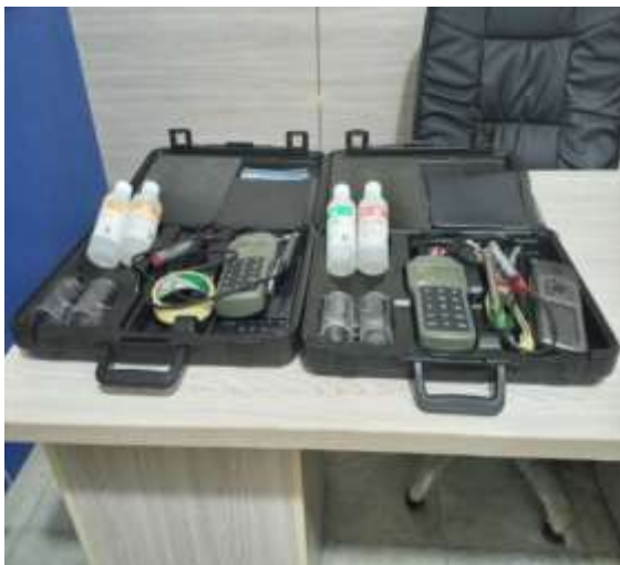
Plate II. HANNA Test kits for measuring pH, TDS and EC
