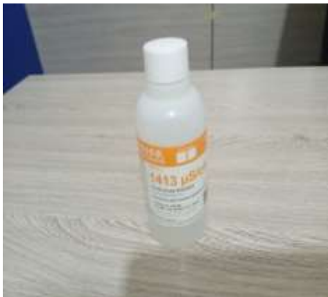
Plate VI: Reagent for calibration of electrical conductivity meter
