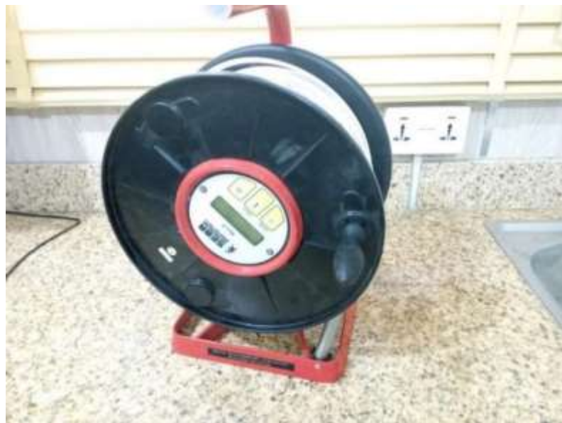
Plate V: Static water level and temperature measuring dip metre
