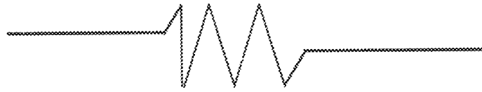
Figure 2.6 Circuit symbol for linear resistors.
