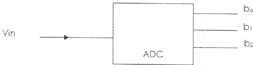
Fig 2.1: Diagram of a 3-bit ADC
