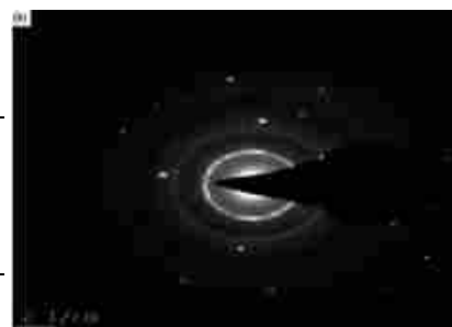
Fig.9: (a) EDS and (b) SAED of Purified Carbon Nanotubes
