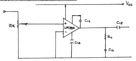
fig 3.1 Audio Amplifier Stage
