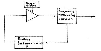
Fig. 2.4 Block diagram of a typical oscillator
