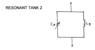
fig 3.4 Tank Resonant
