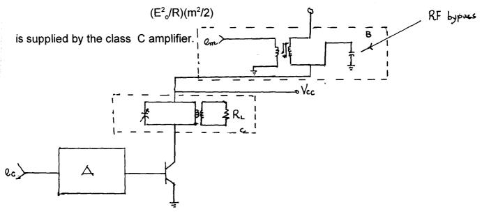
Fig. 2.5 collector-modulated transistor
