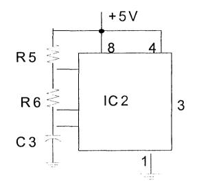
fig 3.3 astable oscillator stage
