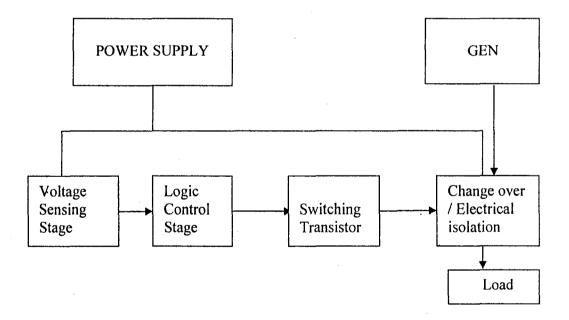
Fig 1.0 Block Diagram of an automatic change over switch
