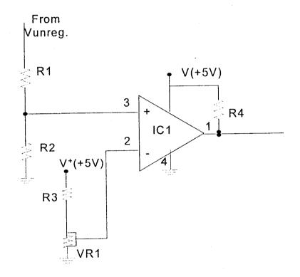
fig 3.2 comparator stage.
