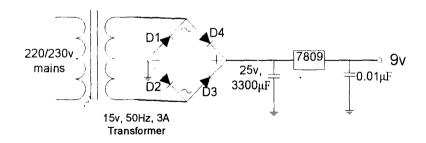
FIG 3.0 Power Rectification Process to 9v
