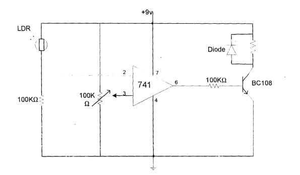
FIG 3.5 The LDR circuit diagram as used in this project.
