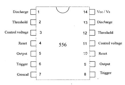
FIG 3.2 Pin Configuration of the 556 Integrated Circuit (IC)
