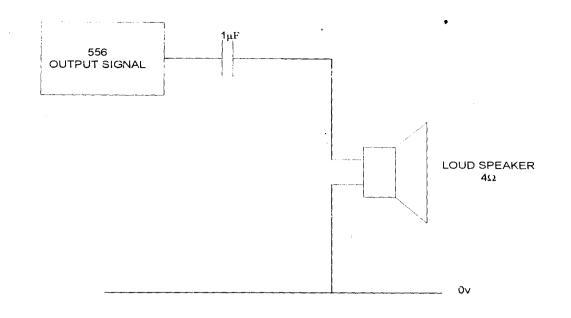
FIG 3.8 Connection of the Siren to the Speaker
