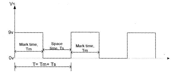
FIG 3.7 Square Waveform Output of a Warbling Siren
