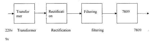
FIG 3.1 block diagram illustrating the sequence of rectification of this project
