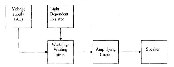
FIG 1.1 Block diagram of warbling-wailing siren with light dependent resistor The warbling-wailing siren is composed of many functional blocks. Each block is a simple circuit with few components. The figure 1.1 shows the block diagram of a warbling-wailing siren, incorporated with light dependent resistor and an alternative voltage supply for back up in the event of power outage.
