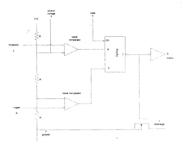
FIG 3.3 General Functional Block Diagram Of The 556 In Astable Mode
