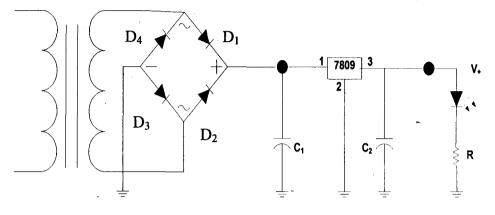
FIG. 3.5 Power supply circuit
