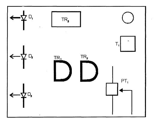
Fig. 4.0 Component layout of the transmitter on vero board
