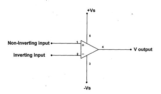
Fig 2.3 Basic operational amplifier symbol
