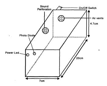
Fig. 4.3 Isometric view of receiver cased with dimensions
