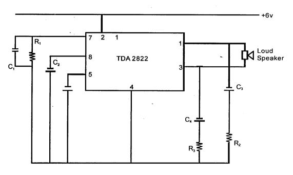
· Fig. 3.4 Output stage circuit diagram
