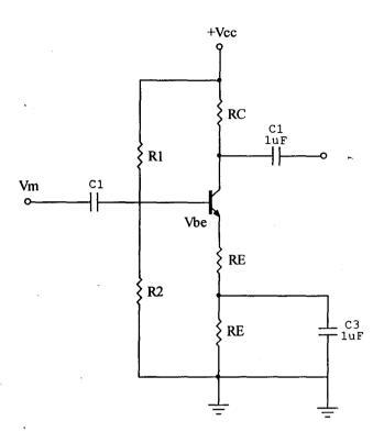
Fig 2.1 Transistor as an Amplifier
