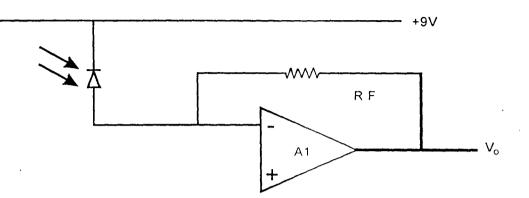
Fig. 3.3 (Photodiode and operational amplifier)
