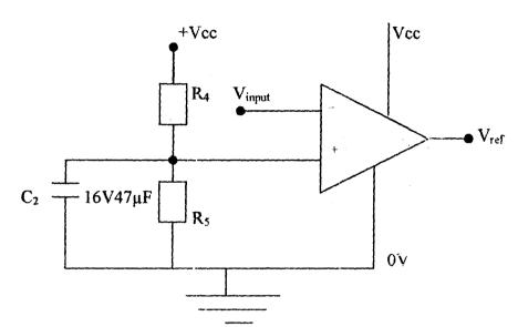
FIG 3.3 SINGLE-SUPPLY BIASING OF AN OP-AMP
