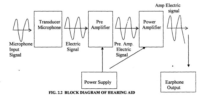
When audio signal is incident or picked up by the microphone, the sound causes acoustic pressure on the microphone. The microphone converts this pressure to equivalent voltage. The microphone output voltage is fed into a broad band amplifier, which preamplifies the voltage signals. The output of the pre-amp is then passed into an amplifier stage before it is passed into a transducer (earphone).
