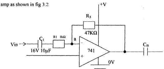
Fig 3.2 741 inverting Op-Amp
