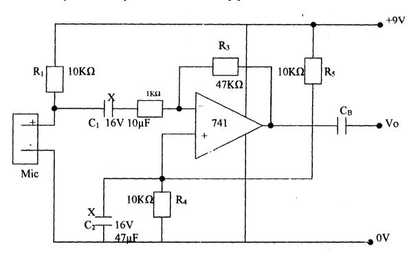
Fig 3.1 Microphone Preamplifier
