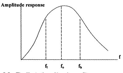
Figure 2-2 The illustration of band-pass filter response.
