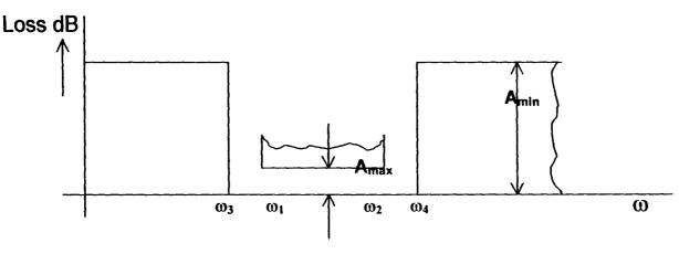
Figure 1-2 Typical band-pass requirements
