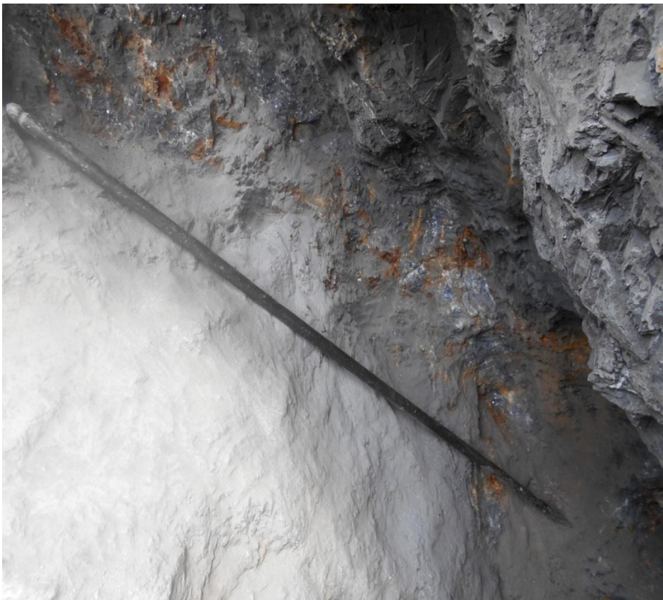
Plate II: Indurated Dark Grey Shales observed in a Lead-zinc Pit at Royal Salt Mining Pit
