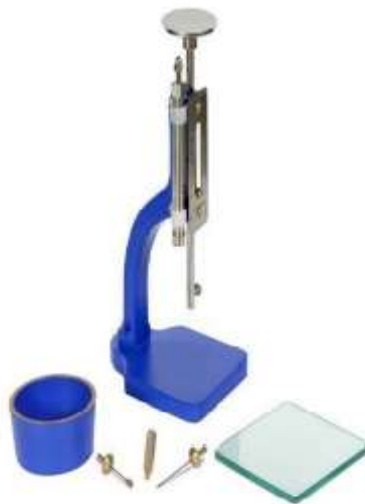
(a) Schematic diagram of a vicat apparatus
