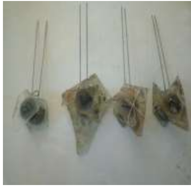
Plate B7: Soundness test sample
