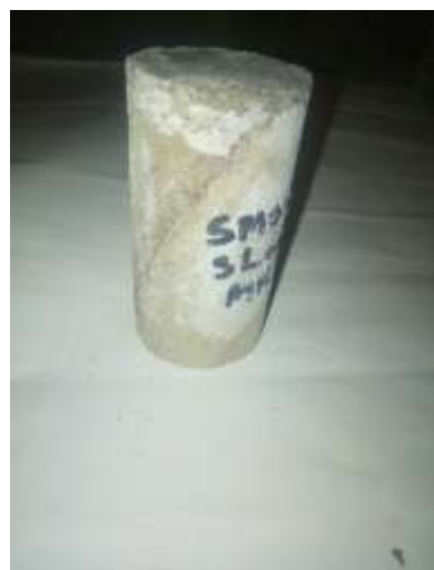
Plate B11: Cylinder splitting Shear bond test sample
