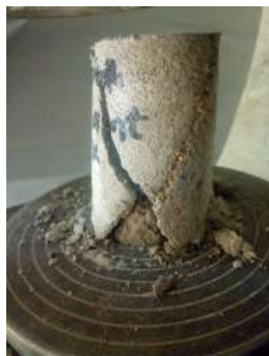
Plate B12: Failure mode of Cylinder splitting Shear bond test sample
