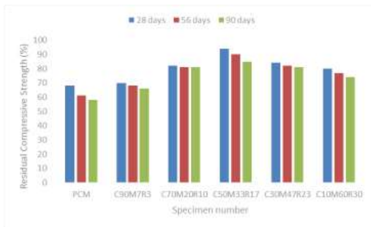
Figure 4.6: Strength losses as caused by H 2 SO 4 attack on ternary blended GPMs
