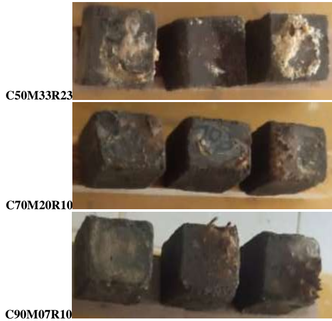
Plate II: Visual appearance of specimen after immersion in H_2SO_4
