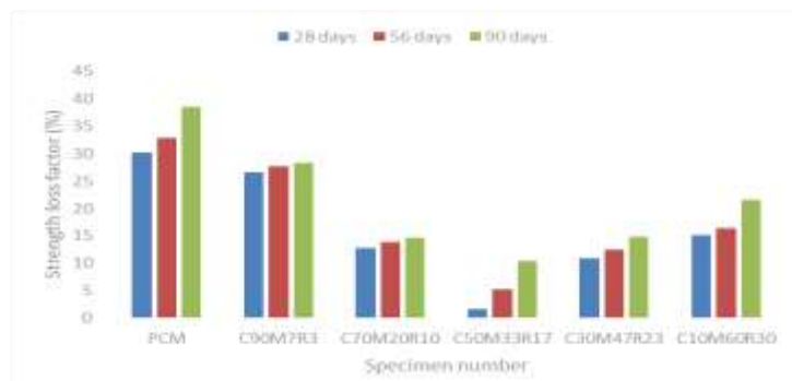
Figure 4.4: Strength loss factor (SLF) of ternary blended GPMs exposed to sulphate solution
