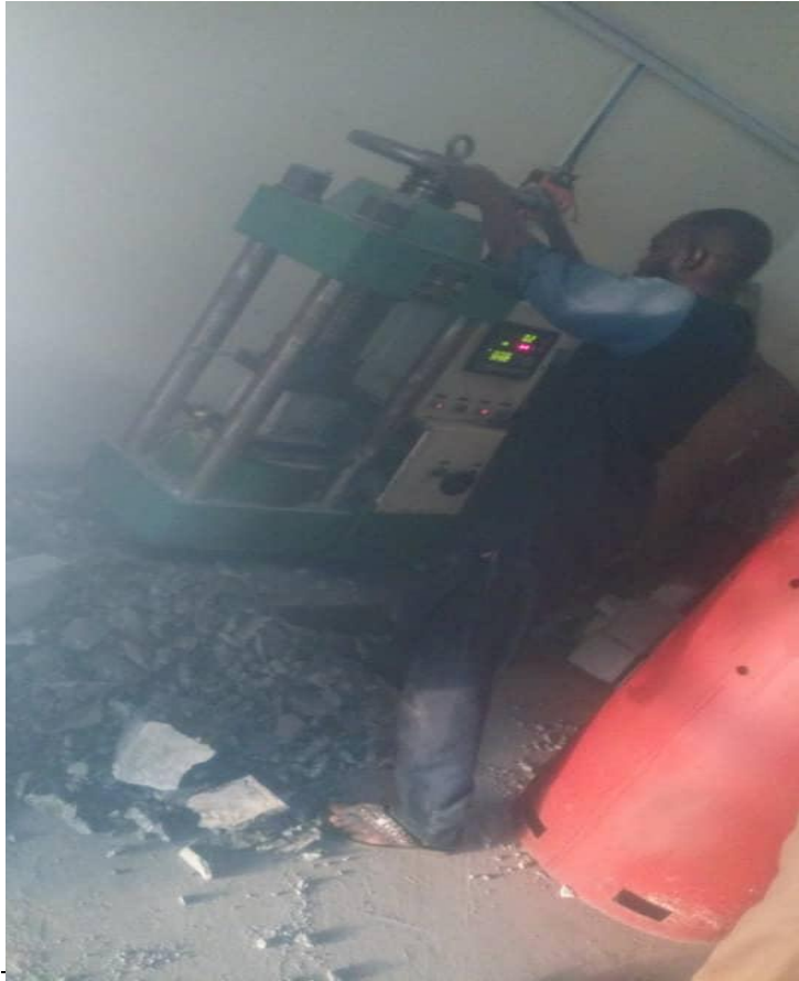
Plate V: Crushing of concrete cubes
