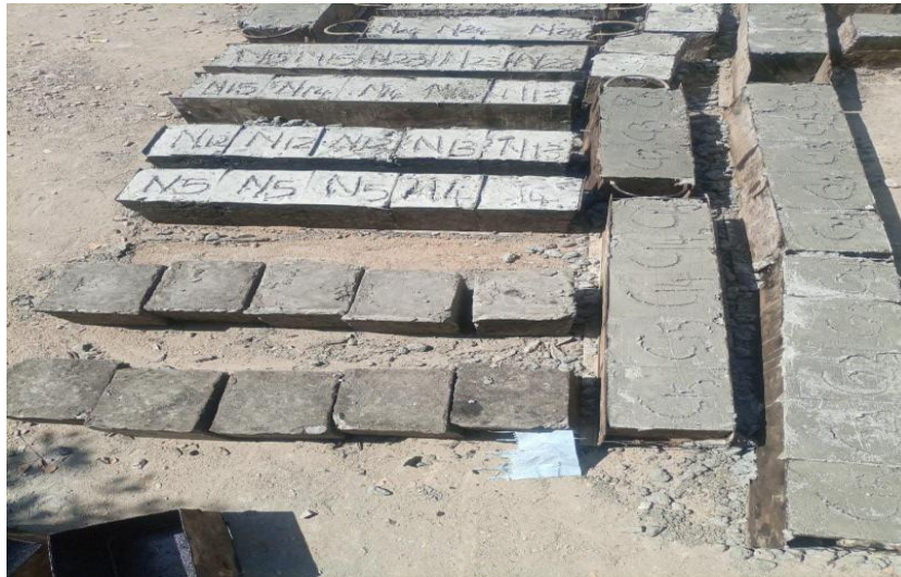
Plate III: Concrete cubes after casting
