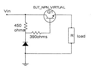
Figure 3.4: Series regulation circuit
