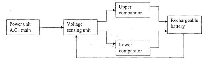
Figure 3.1: Block diagram of the circuit
