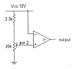
Figure 3.7: Lower comparator of the 555 timer
