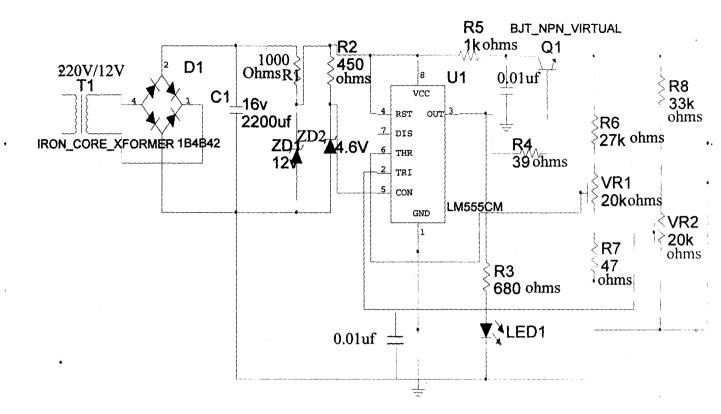
Fig. 3.9: Complete circuit diagram of a Nokia 1200 cell phone battery charger
