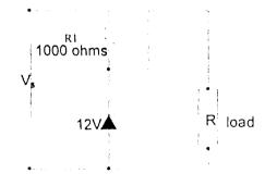
Figure 3.3: Diagram of a voltage regulator
