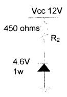
Figure 3.5: Diagram of a reference voltage
