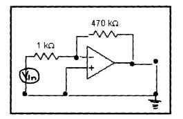
FIG.2.2.1 INVERTING AMPLIFIER
