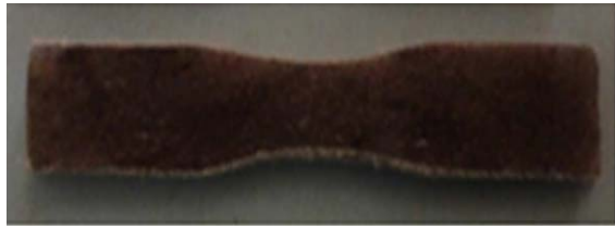
FIG. 1. A typical samples produced and machined as a specimen for tensile testing. [Color figure can be viewed in the online issue, which is available at wileyonlinelibrary.com .]
