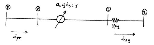
fig. 2.1.7 Phase shifting transformer representation.
