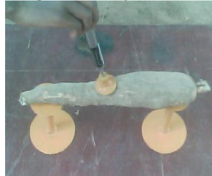
Figure 6: Determination of bioyield force The peeled cassavas with the developed tools are shown in Figure 7.
