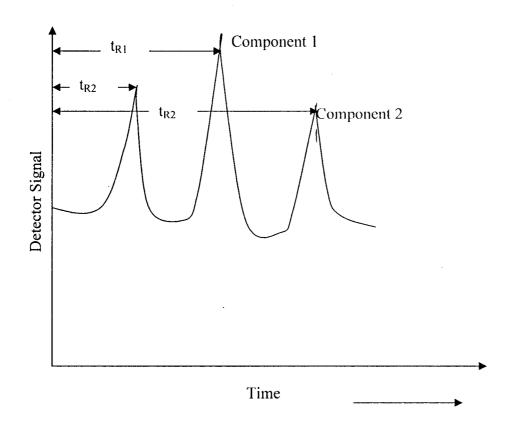
**Fig. 2.2** Gas chromatograph for a two – component system in the liquid phase is extremely low (oxygen or air) for example. It rate of movement will approach the rate of flow of the carrier gas and solid phases, note the air peak in the figure above.
