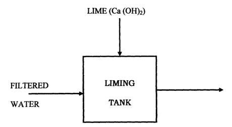
This unit helps to increase the pH of the water to 7 due to the acidity of the water from the filtration tank. The dosage of the lime added is determined by laboratory test. The liming process also helps to remove hardness of the water by dissolving the calcium as magnesium ions are present in the water.
