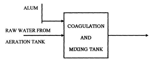
Coagulation is the driving together of colloidal particles by chemical forces. This process is speedy and occurs within seconds of the application of a coagulating reagent (alum) to the aerated water. For this reason, intense mixing is necessary at the point of chemical application in order to assure uniform chemical distribution and exposure of fine particles in the water to the coagulating agent before the coagulation reaction is completed. However, this is the work of rapid mixing.
