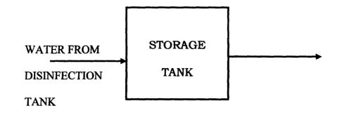
The final storage tank is the tank or container where the purified water is been kept for use (for different domestic purposes).
