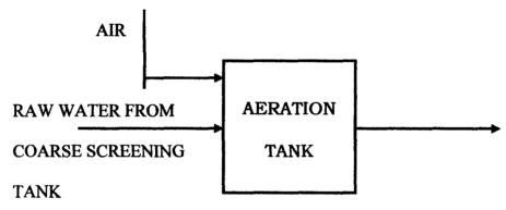
As it is applied to domestic waste water treatment, aeration can be defined as the process by which a gaseous phase usually air and water are brought into intimate contact with each other for the purpose of transferring volatile substances to or from the water. These volatiles substances include oxygen, carbohydrate, nitrogen, hydrogen sulphate, methane and various unidentified organic compounds responsible for taste and odour. The purposes of this unit are as follows:
