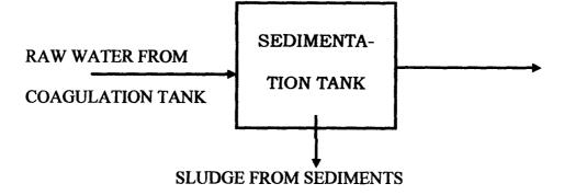
This process unit is used to reduce the amount of settleable solids by chemical treatment, such as the addition of coagulant to remove colour and turbidity, this unit is
