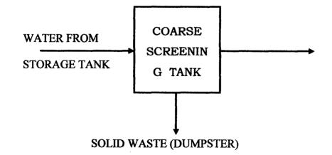
This is a primary process used to remove larger entrained objects ranging from 100 - 1000 mm in size that are deposited in the waste water tank, such as rags, sticks,
