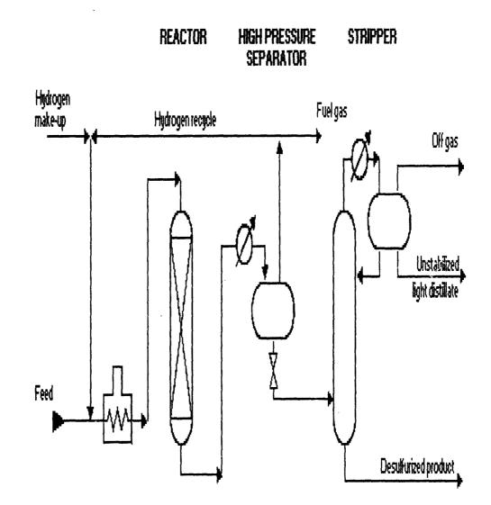
FIGURE 2.2: FLOW DIAGRAM FOR HYDROTREATING PROCESS
