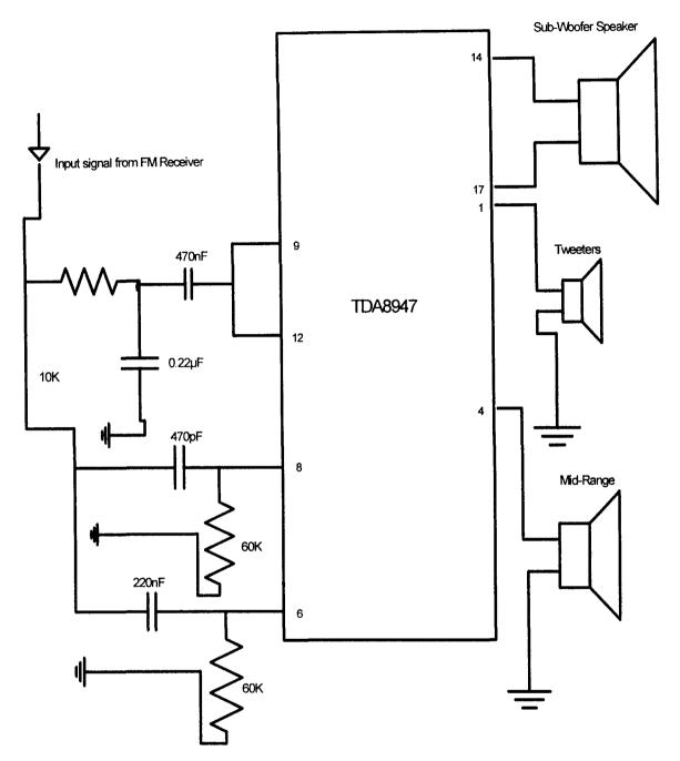
Fig. 3.6 Pin connection of the Power Amplifier to the loud speakers
