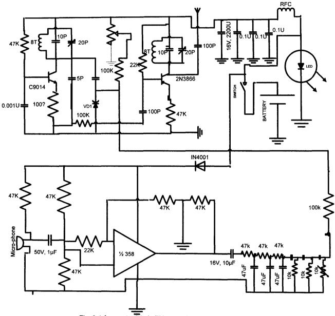
Fig. 3.4 A varactor Diode FM transmission circuit
