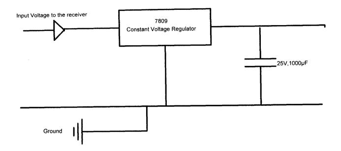
Fig.3.3 FM Receiver's power supply
