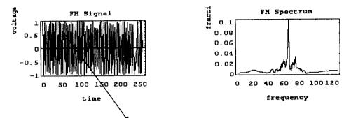
fig. 2.3 A frequency spectrum within a specified band width
