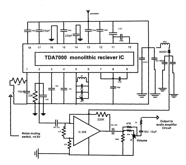
Fig.2.7 Circuit diagram of a TDA 7000 Frequency Modulation Receiver (all ground connection should terminate at pin 16)
