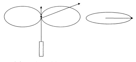
Radiation in the vertical plane b. Radiation in horizontal plane
