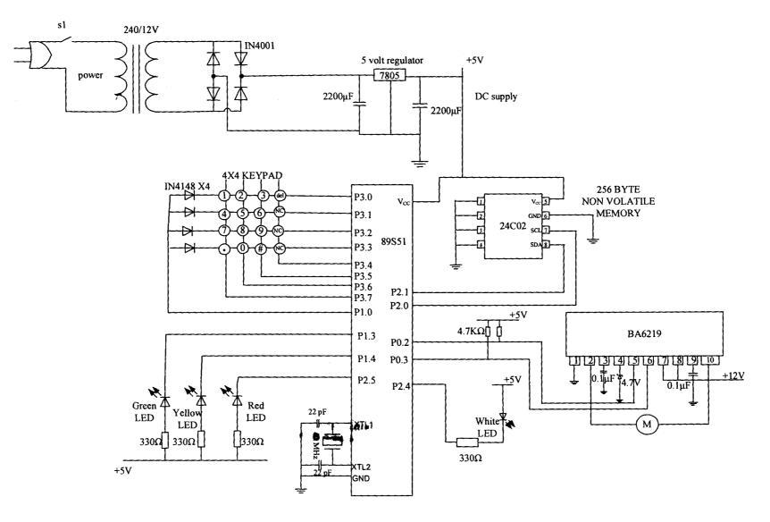
Fig.3.8 ELECTRONIC SECURITY KEYPAD LOCK
