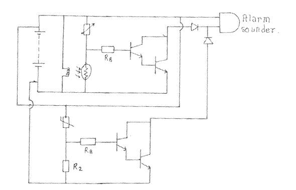
Fig. 2:3.1 a CIRCUIT DIAGRAM OF THE SMOKE AND HEAT DETECTOR
