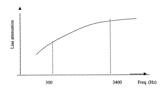
Fig.2.2(a) Attenuation Frequency characteristics.
