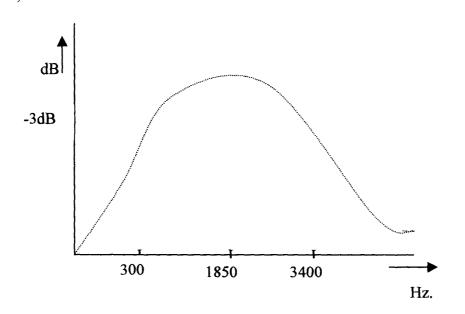
Fig. 2.2 (E) Frequency response of the band – pass filter.
