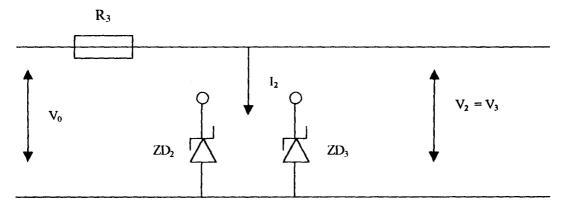
Fig 2.1 (e) Shunt regulator- (voltage).
