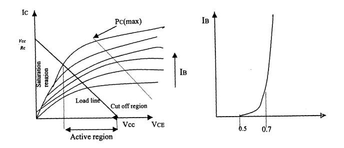
Fig.2.1 (b) Output characteristics with load line fig 2.1 (c) input characteristics A plot of  $I_B$  versus VBE interrelates the two input parameter as the device input characteristics shown in fig 2.1 (c)
