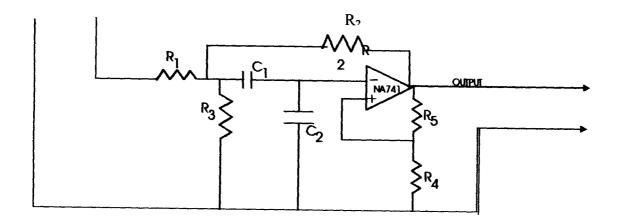
Figure 2.2(1) Band pass filter circuit.
