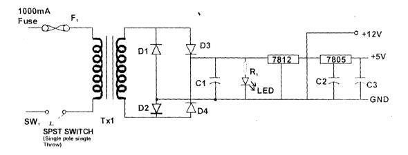
Fig. 3.2. Power supply circuit.
