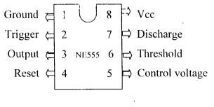
Fig. 3.3. Showing symbol of the 555IC
