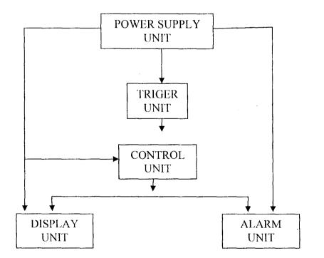
Fig. 3.1 Block diagram of four-door monitoring alarm system
