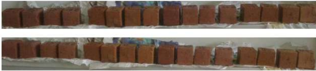
Figure 3.2 Prepared test samples (laterite bricks)
