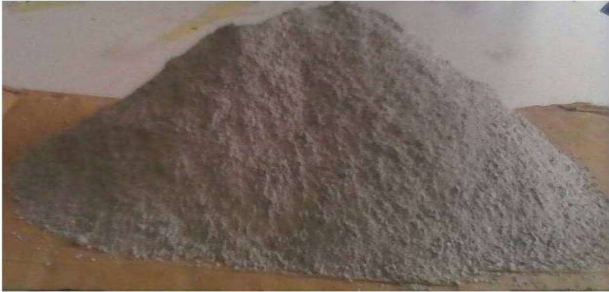
Figure 3.1 (c): Cattle bone ash after calcination and grinding
