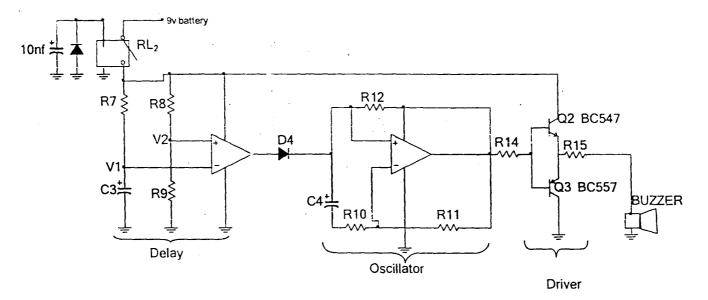
Fig 3.8 CIRCUIT DIAGRAM OF MAINS FAILURE ALARM
