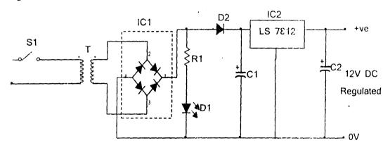
fig 3.2: 12v de regulated power suppLy circuit design
