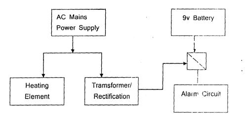
Figure 2.5: block diagram of power distribution in incubator
