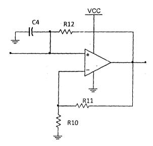
Fig. 3.6 Oscillator Circuit
