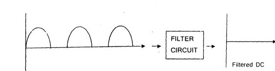
Fig. 2.4 Diagram of a Filter Function
