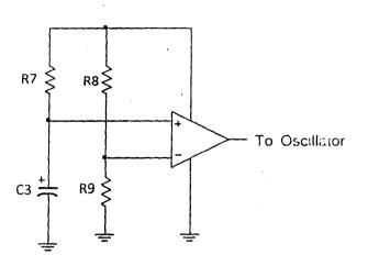
Fig. 3.5 Time delay Circuit
