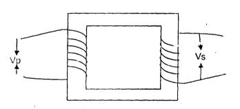
Fig 2.2 Diagram of a Transformer
