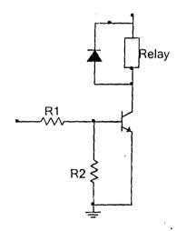
Figure 2.8: switching circuit of the egg incubator
