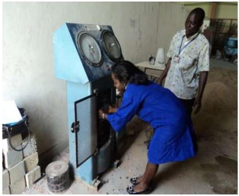
Taking reading of the crushing load
