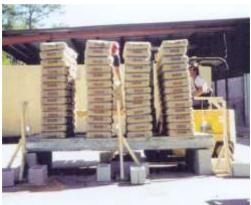
An EPS slab being tested via axial loading in Mbora district.
