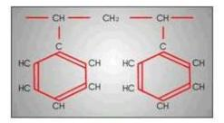
The above is known as poly(1- phenylethene-1,-2-diyl), it has a density of  $1.06 \text{kg/m}^3 - 1.12 \text{kg/m}^3$ , thermal condition of 0.033 w/m.k and a refractive index of 1.6.
