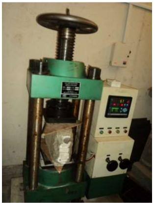
An EPS block being crushed with a crushing machine.
