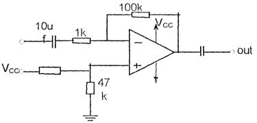
Fig. 3.3 showing the connection for the pre-amplifier stage.
