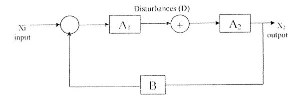
Fig. 2.11 showing the unwanted effect in amplifier.
