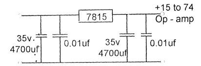
Fig. 3.2 Showing regulation unit connections.
