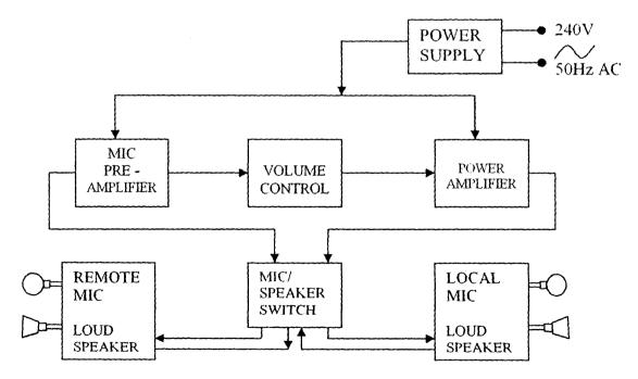
Fig 1.1 BLOCK DIAGRAM OF A SINGLE CHANNEL INTERCOM SYSTEM
