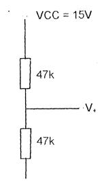
Fig. 3.4 showing the biasing arrangement of the pre-amplifier stage.
