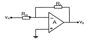
Fig. 2.7 Showing an operational amplifier as a sign changer.
