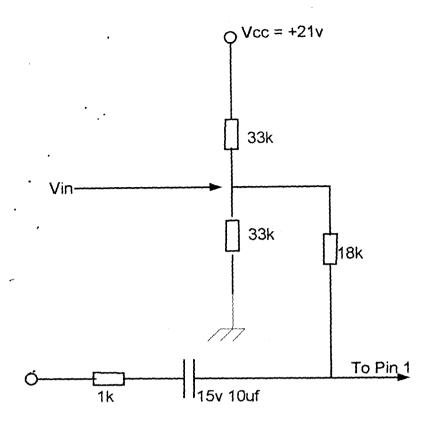
Fig. 3.8 showing the biasing arrangement.
