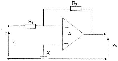
Fig. 2.3 Inverting operational amplifier.
