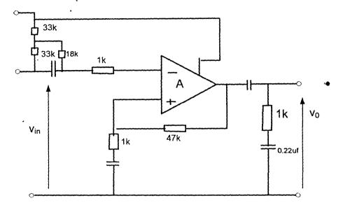
Fig. 3.7 showing the power amplifier unit arrangement.
