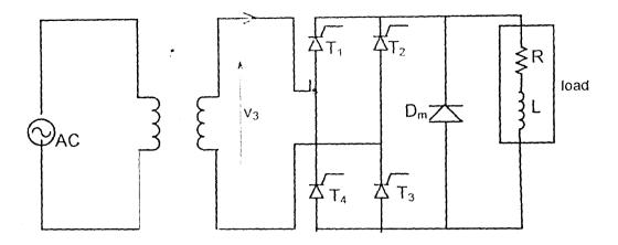
Fig 2.13a Shows a Bridge Converter Circuit.
