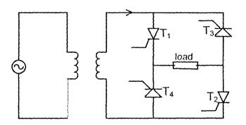
Fig. 2.12a Showing a Bridge Full wave Connection.
