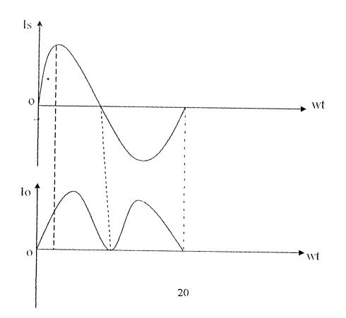
Fig. 2.12d showing the output wave forms of a full wave rectifier.
