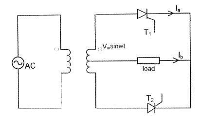
Fig. 2.12b Show a Bi-phase full wave connection.
