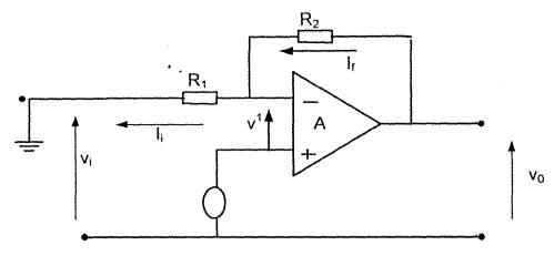
Fig. 2.6 Showing non – inverting operational amplifier connection.
