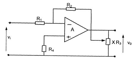
Fig. 2.4 showing the gain of the inverting amplifier.
