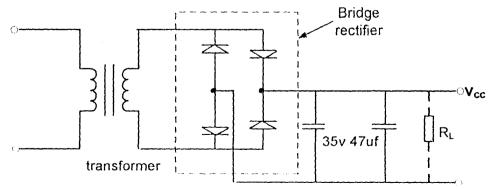
Fig 3.1 The power supply unit of the design.
