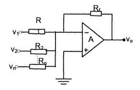
Fig 2.10 Showing op-amp as an adder or summing amplifier.
