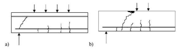
Figure 2.1 Possible shear fatigue failure modes in beams without stir ups
