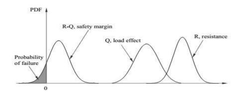
Figure 2.2: Probability Density Function of load, resistance, and safety margin(David, 2010)
