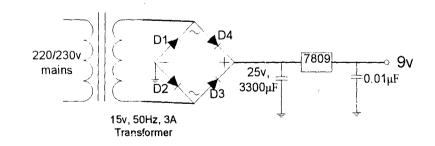
FIG 3.0 Power Rectification Process to 9v
