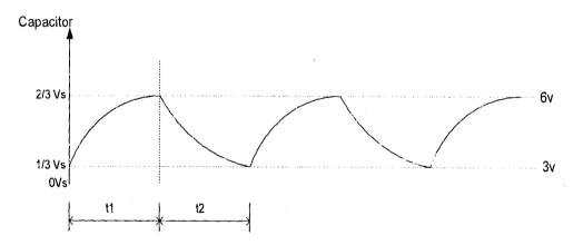
FIG 3.6 The Wailing Output Waveform of the Siren
