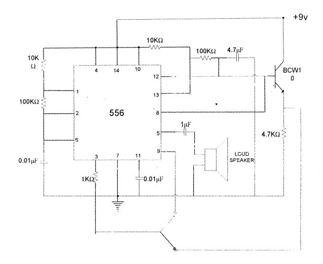
FIG 3.4 The circuit symbol with its connections for this project The astable circuit of the 556 produces square waves [6]. This is a digital waveform with sharp transition between LOW (0v) and HIGH (+Vs).
