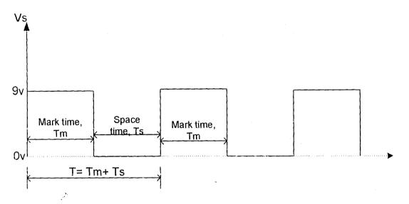
FIG 4.1b Graphical Representation of the Siren Output
