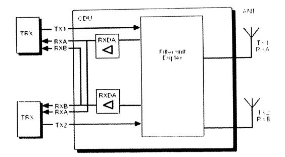
Figure 3.5.2 BLOCK DIAGRAM OF RBS 2302
