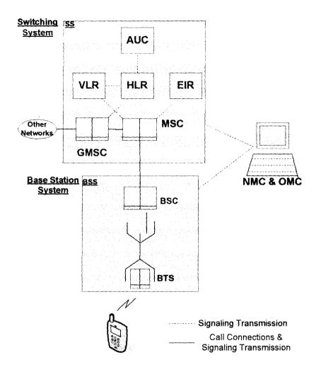
Figure 2.3.1: GSM Network Component
