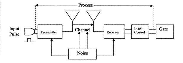
Fig 2.4 Pulse Transmitter
