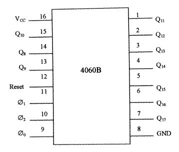
Fig 3.2 Pin Assignment of 4060B
