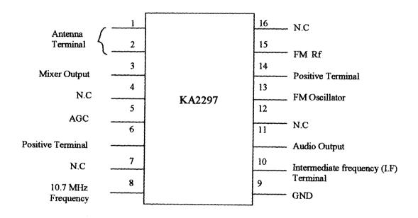
Fig 3.4 Pin Connection of KA2297
