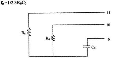
Fig 3.1 frequency Output of 4060B
