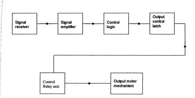
Radio Remote Control Circuit. Block Diagram
