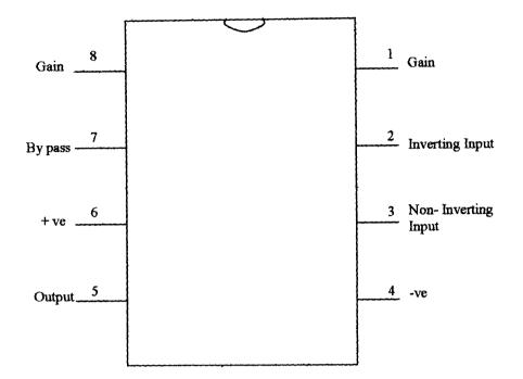
Fig 3.6 Pin assignment of LM 386
