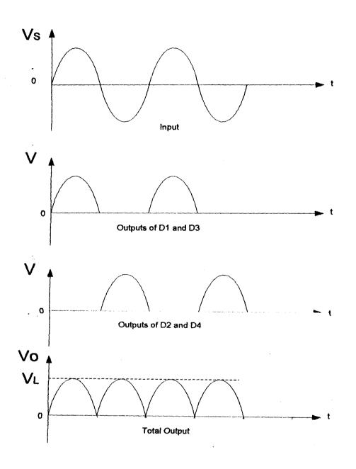
Fig. 3.5: wave diagrams of full- wave rectification process
