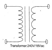
Fig. 3.2: (a) A transformer circuit symbol
