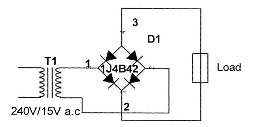
Fig. 3.3 Schematic diagram of rectifier circuit
